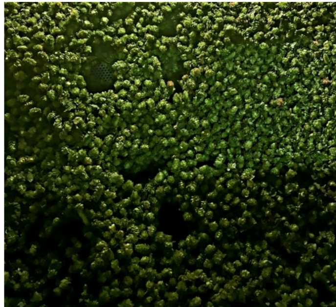
Figure 7. Air channel formation in a 15 kg/m 2 bulk of hops.
