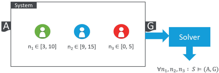
Fig. 7.3. System Verification: Given a system contract (A,G), a set of component types, and their allowed amounts in the system, prove that any possible combination of components fulfils the contract.
