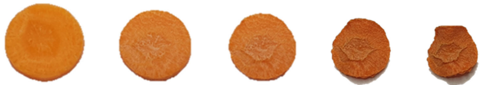
Fig. 5 Changes in carrot sample during drying process (strategy A, 70 °C)
