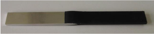
Figure 4: Sample designated for the mechanical examination of the adhesive properties
