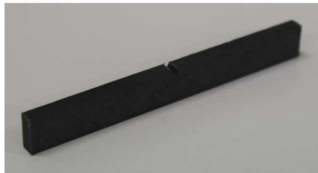
Figure 3: Charpy sample designated for the mechanical examination of the basic material properties
