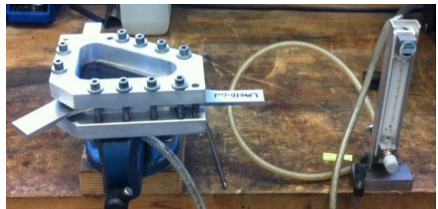
Figure 8: Testing unit for the measurement of the flow of a leak and for the identification of unsealed areas
