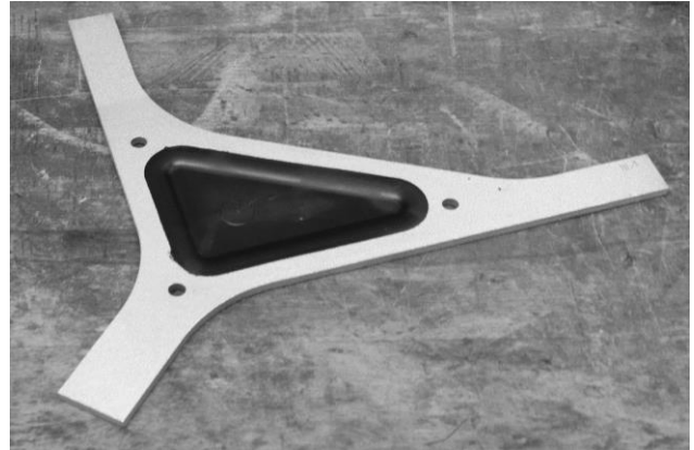
Figure 6: Hybrid samples that were similar to models used in practice, and were designated for the examination of the sealing of the composite
