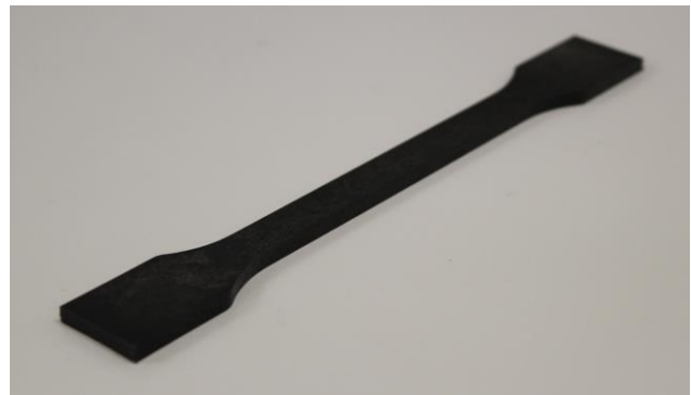
Figure 2: Tensile test sample designated for the mechanical examination of the basic material properties
