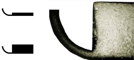
Figure 5: Cross-section of a specimen manufactured using the pull and foam – method, core movement of 2mm to 8mm (personal preliminary investigations), right: specimen with fine pore distribution
