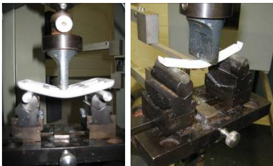
Figure 3: 3-point-bending test on component (left) and extracted plank (right)
