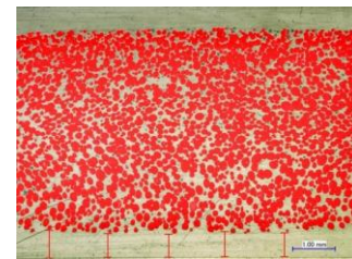
Figure 6: Morphology of thick-walled section with pore ratio of up to 68% and a marginalised layer thickness of approx. 0,6mm
