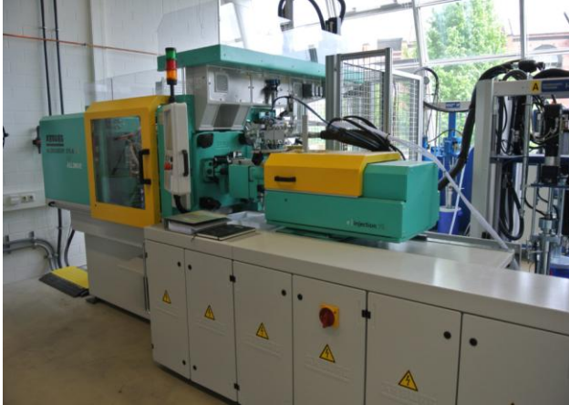
Figure 5: Arburg Allrounder 370A 600-70/70 multicomponent injection molding machine with robot system
