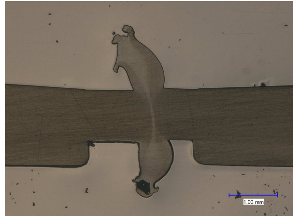
Figure 10: Light microscope image of a polypropylene sample with 20mm diameter and a wall thickness of 1mm
