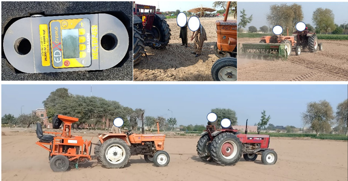
FIGURE 7 Power measurement in field through dynamometer.
