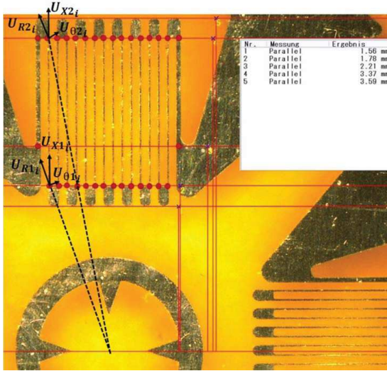
Figure 3.4 Strain gauge type EA-062RE and active parts of a strain gauge grid.
