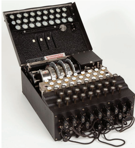
FIGURE 2.5: Military Enigma machine, model “Enigma 1”
