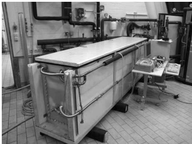
Fig. 4. Test station for heat exchanger samples
