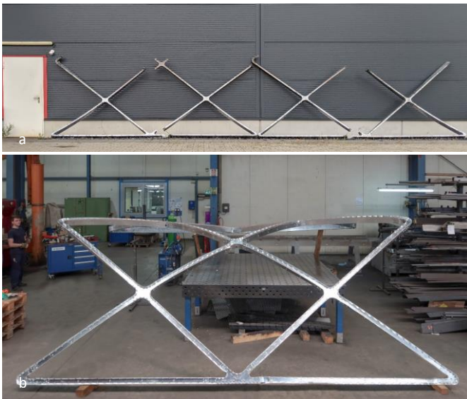
Figure 12: a) Hot dip galvanized 4 sets, b) Off-site assembly.
