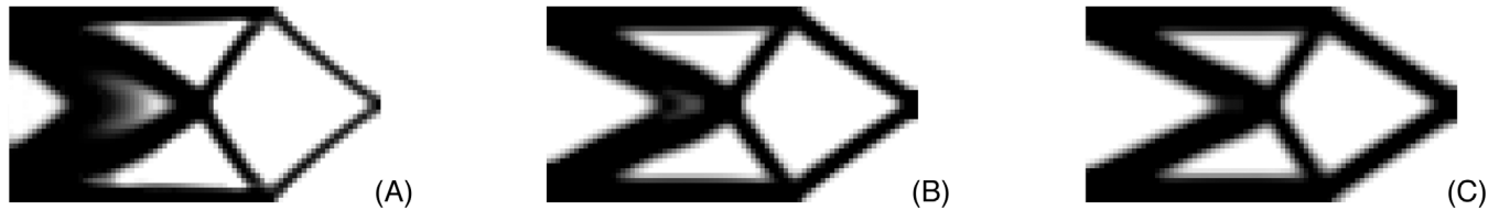
FIGURE 8 Result of cantilever beam for combined loading by external force and self-weight with (A) \frac{F}{F_0^g} = 0.2 and (B) \frac{F}{F_0^g} = 1 and (C) \frac{F}{F_0^g} = 6 .
