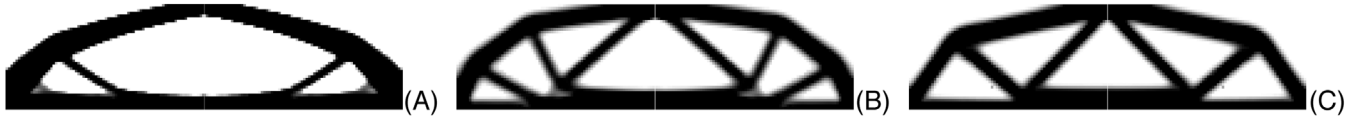
FIGURE 6 Result of MBB beam for combined loading by external force and self-weight with (A) \frac{F}{F_0^g} = 0.2 and (B) \frac{F}{F_0^g} = 1 and (C) \frac{F}{F_0^g} = 6 .
