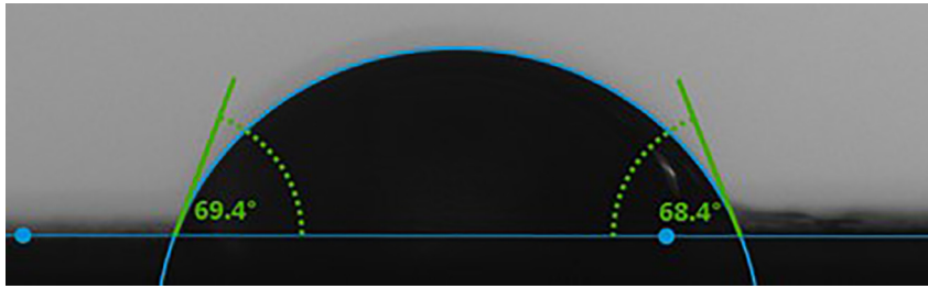
Figure 3: Two three-phase angles of a water drop on a PLA blend substrate surrounded by air.
