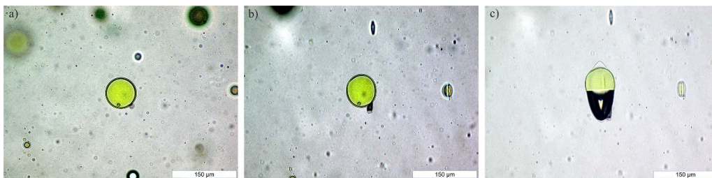
Figure 12. Example of capsule elongation in (a) initial condition, (b) at 100% and (c) 150% Cauchy strain of the surrounding elastomeric matrix.
