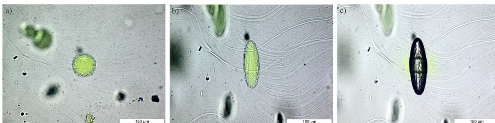
Figure 13. Example of capsule bursting in (a) initial state, (b) at 100% and (c) over 100% Cauchy strain of the surrounding elastomeric matrix.
