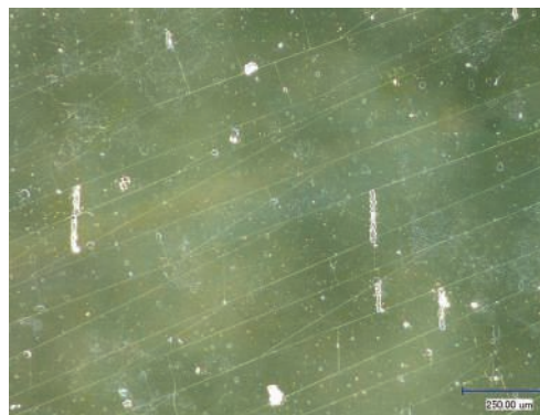
Fig. 7. Example of cracks on ITO layer without bending (after ageing), 200x
