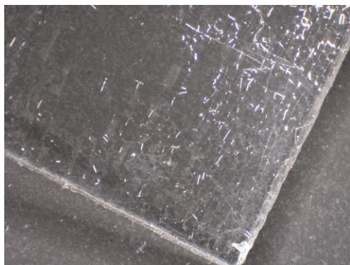
Fig. 5. Degradation at the TiO 2 surface (magnification: x21)
