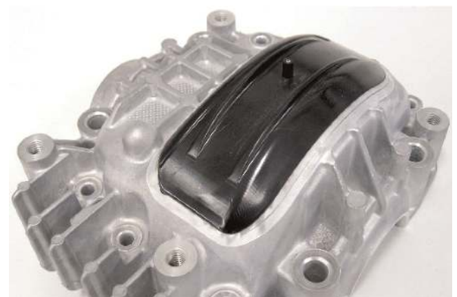
Fig. 13. Final hybrid gear housing demonstrator
