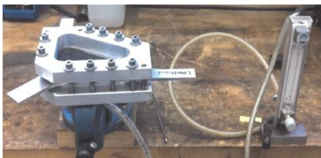
Fig. 10. Experimental setup for tightness testing
