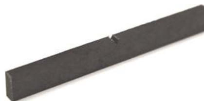
Fig. 3. Charpy test specimen notched acc. to DIN EN ISO 179-1, type 1-B for mechanical examination of basic material properties after media exposition
