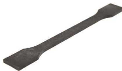
Fig. 2. Injection-molded tensile test specimen acc. to DIN EN ISO 3167 for mechanical examination of basic material properties after media exposition
