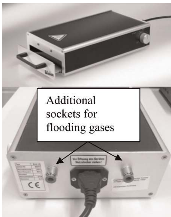
Fig. 1. UVC chamber with additional sockets for flooding in gases (Dinies Technologies GmbH, Villingendorf, Germany)
