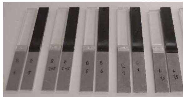
Fig. 10. Metal-plastic specimens with polycarbonate (transparent) for demonstration and polyamide (black) for tensile tests
