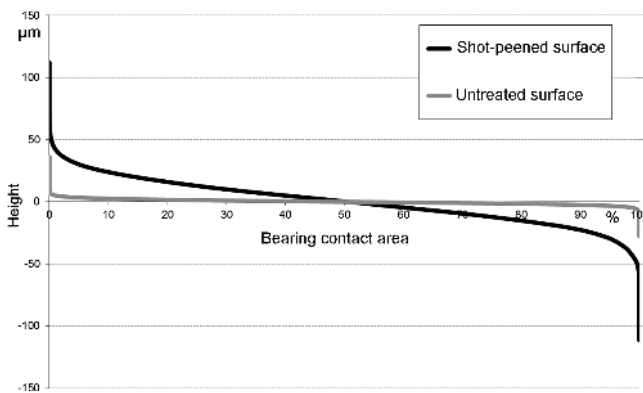
Fig. 5. Bearing area curves of a untreated aluminum surface and a shot-peened aluminum surface
