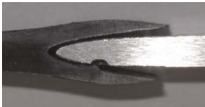
Fig. 12. Fracture behavior of 1 mm lens geometry with shot-peened surface
