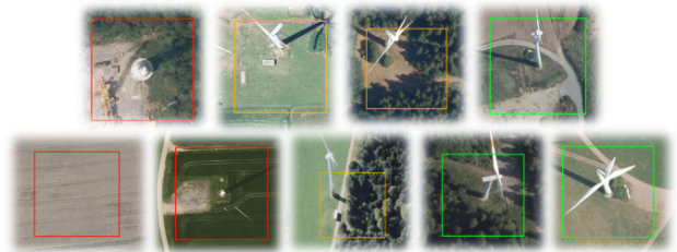
Fig. 2. Samples based on their suitability for training. The images marked in red are unsuitable due to incorrect position or poor image resolution, the images marked in yellow contain wind turbines that are clearly visible but were rejected for fine-tuning due to their inaccurate position. The images marked in green contain turbines whose tower base is located directly in the center of the respective boxes.
