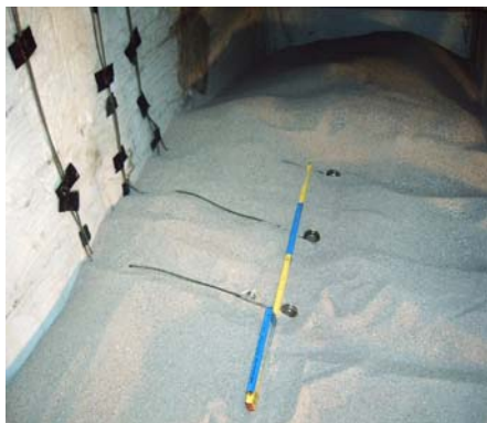
Figure 3.5: Positions of the horizontal earth pressure cell
