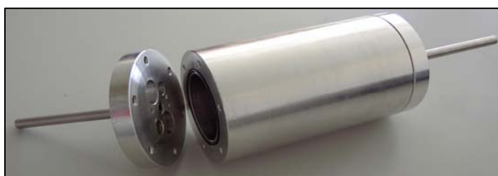
Fig. 45. A versatile gas flow cell for single cantilever investigations.
