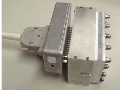
Fig. 57. Pre-amplifier attached to the cantilever cell.
