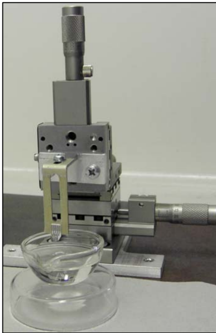
Fig. 81. Cantilever functionalization by dipping into polymer solution.
