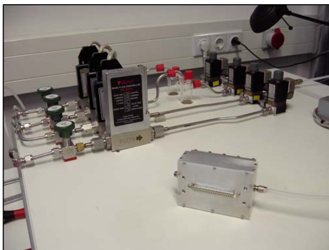
Fig. 54. The cantilever cell operating in gas flow mode.
