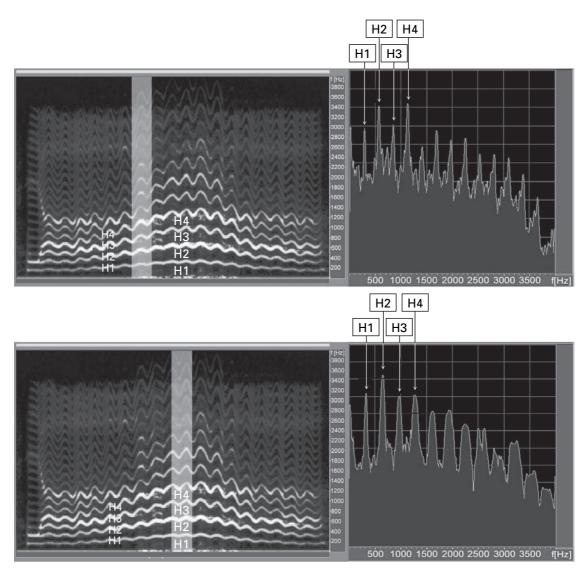
**Fig. 2.** Sonagrams (left) and amplitude spectra corresponding to the light vertical stripes in the sonagrams (right) of the same scale as shown in figure 1 but sung *without* register transition. In the top row  $H_2$  and  $H_4$  are strong again. On higher pitches (bottom row),  $H_2$  remains the strongest harmonic.
