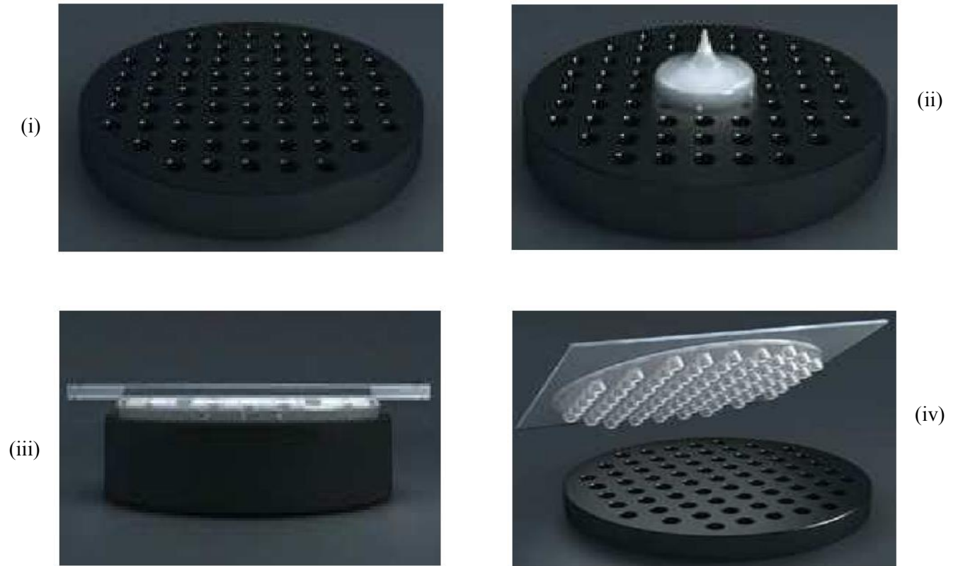
Fig. 5.6 Schematic of SCIL template replication process: (i) Deposition of anti-adhesive layer on the master template, (ii) Dispensing of PDMS: h-PDMS is coated and s-PDMS is poured, (iii) Positioning of the glass carrier on the master template coated with PDMS and curing of PDMS at 50°C on MRT, (iv) Separation of the master template and the glass carrier [107].
