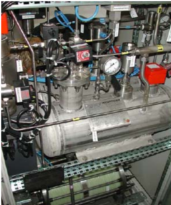
The alkaline Electrolyser 3.6kW (Hydrogen Systems) and the PLC Box from Hydrogen Systems, www.hydrogensystems.be
