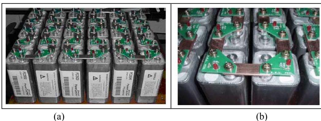
Fig. 3.11: (a) Supercapacitor module; (b) An enlarged photograph of (a) [Schneuwly-02].
