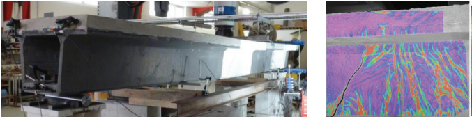
Figure 2: Specimen at bearing load (left) and corresponding bending cracks (left) from measurement with the digital image correlation system
