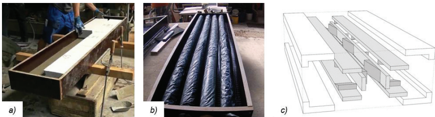
Figure 1: manufacturing methods of the hollow cross sections, a) mineral foam core, b) compressed air filled tubes, c) mechanically expendable wooden formwork
