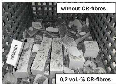
Figure 1: Picture of UHPC specimens after thermal treatment (500°C). Failure under thermal stress without CR-fibres (back row).
