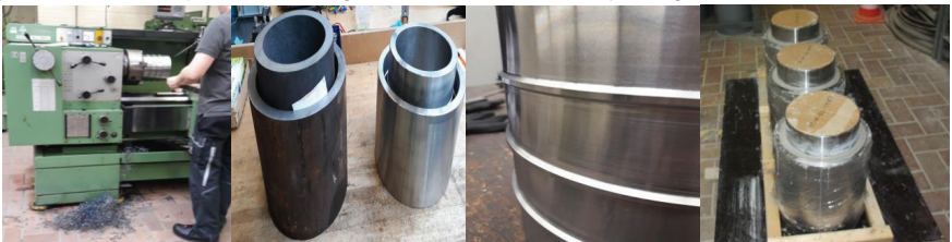
Figure 2: The specimens during the fabrication and after pouring the concrete.
