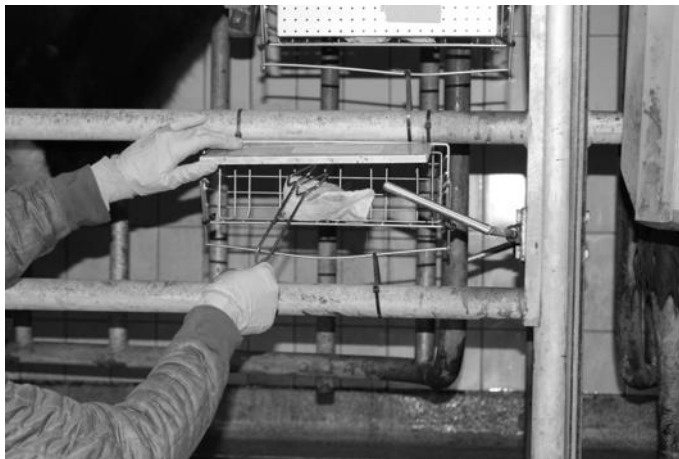
Figure 2: Placing a cloth bag with calf hair in the lower basket with tongs (Source: Kerstin Hofmann)
