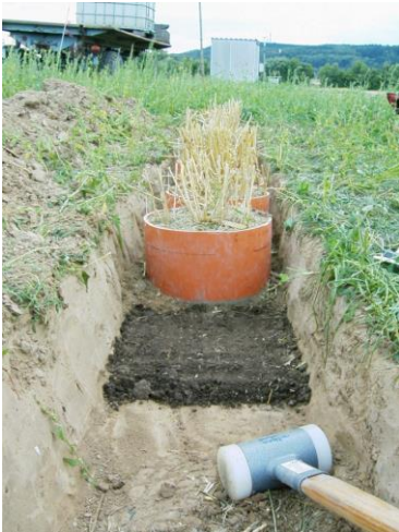
Fig. 1.1. Insertion of 48 columns from four sites and three treatments at the experimental station of Uni Kassel in Neu-Eichenberg.
