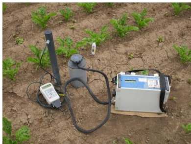
Fig. 1.4. Biweekly measurements of soil respiration, temperature and volumetric water contents in the Friemar site; here in the culture of sugar beet.
