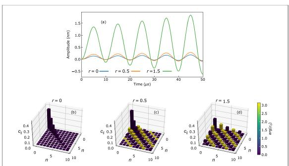
**Figure B1.** (a) Amplification of the axial oscillation amplitude by squeezing the working medium after interaction with both baths. The simulations are performed with  $T_{\rm h}=0.11\,{\rm mK}$  and  $T_{\rm c}=0.1\,{\rm mK}$ . The blue, orange, and green curves represent the trajectories for r=0,0.5 and 1.5, respectively. (b)–(d) Excerpt of the density matrices after interacting with the hot bath and the squeezing operation, where the color encodes the phase of the entries  $\arg(c_{ij})$ .
