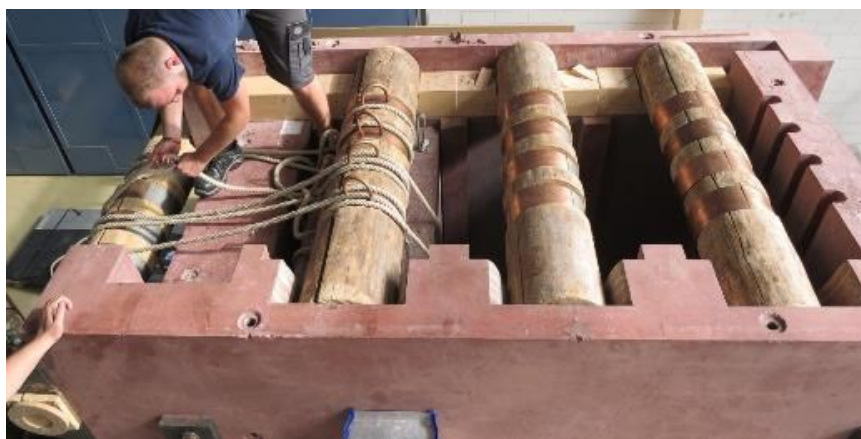
Fig. 4. Top view of the antechamber replica with the south wall to the right. The northern portcullis (N-block) is in its topmost position sitting on a timber beam (fig. 5) while a test is prepared. Note the rounded-out timber wedges on the flat recess of the east wall that provided proper bearings for the logs. (photo by A. Klarendic)
