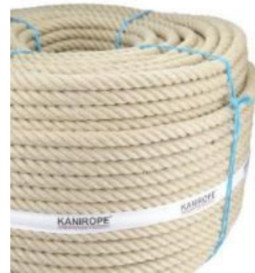
Fig. 7. Twisted halfa grass rope in a sophisticated configuration found with Cheops’ sun bark (left, photo by U.E. Dorka) and diameter 20 mm 4-strand twisted hemp rope used in the tests (right, from KANIROPE product description)
