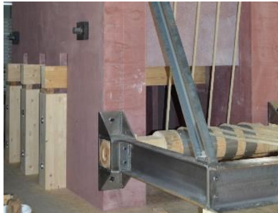
Fig. 5. North entrance of the replica with timber beams placed underneath the portcullises for safe handling during test preparations. The beams were removed just prior to testing. Note the end plates of two steel rods (out of four) that connect the prefabricated concrete elements. The steel frame and log in front are part of the force measurement system. (photo by C. Nguyen)
