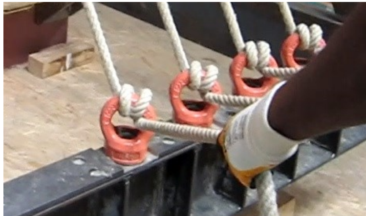
Fig. 3. Rope setting during trials to develop a suitable rope control device. The measurement system is removed so that the controller (here a double loop in the red hoop) receives the full force. (photo by C. Nguyen)
