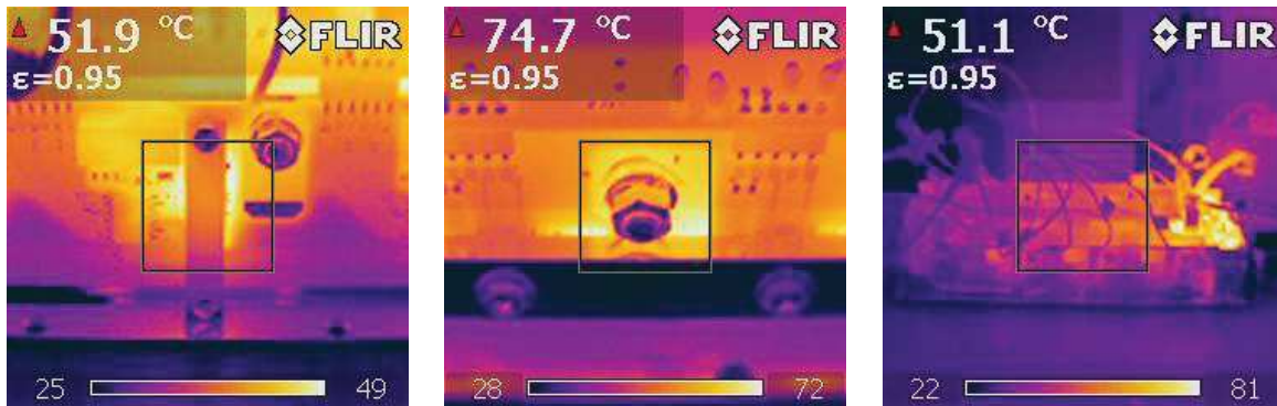
Fig. 12: Worst-case temperatures on the HV GaN switch located on the PCB bottom and measured from the PCB top (left), on the LV switch located under an aluminum hold-down device on the PCB top (middle) and on the complete system viewed from the HV lateral side (right)
