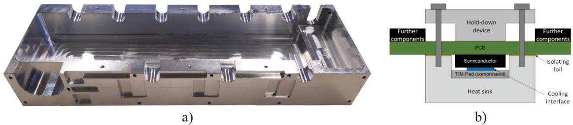
Fig. 6: a) Details of the cavities on the water cooling heatsink and b) schematic cross-section view of a GaN semiconductor mounted in a cavity (not to scale)
