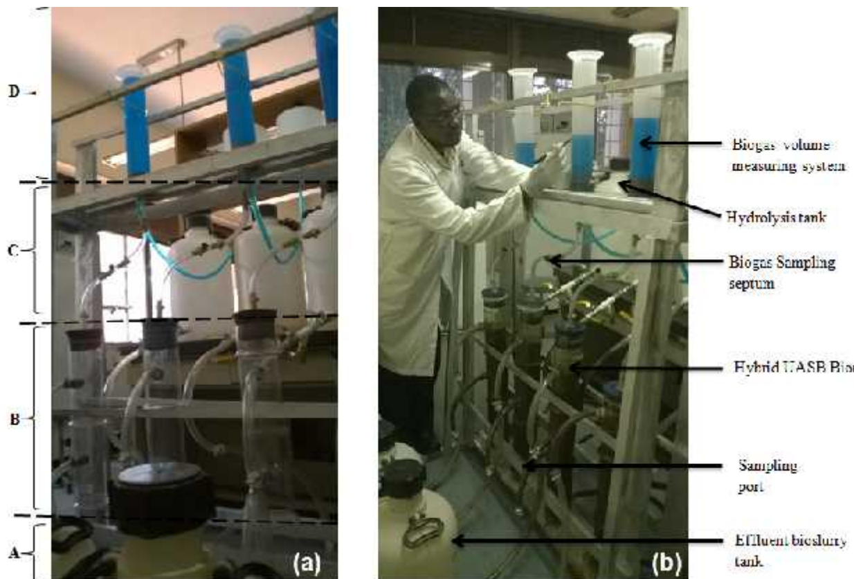
Figure 5.2. Experimental set-up of hybrid UASB bioreactor system
