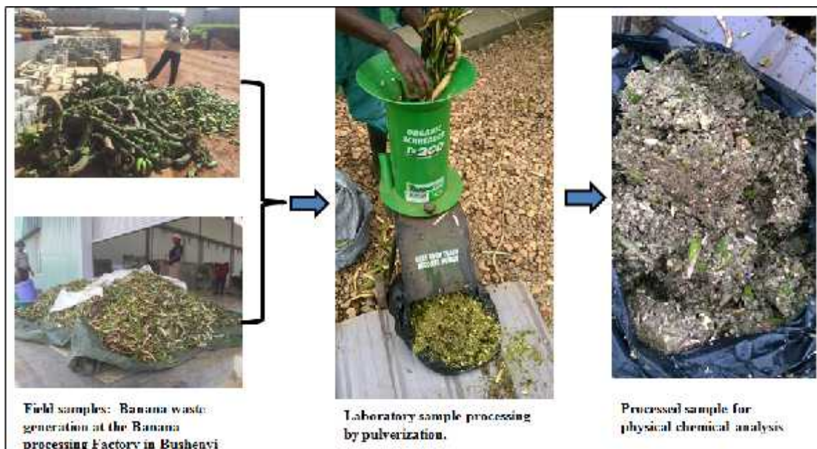
Figure 4.2. Sample preparation for physico-chemical analysis and feedstock for anaerobic digestion
