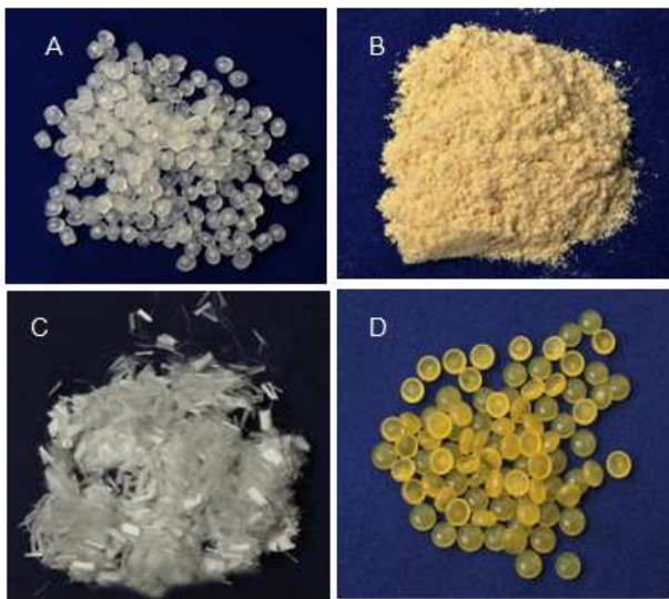
Figure 1: Utilized materials (A: Polypropylene; B: Wood fibers; C: Polyethylene terephthalate fibers D: Bonding-agent)
