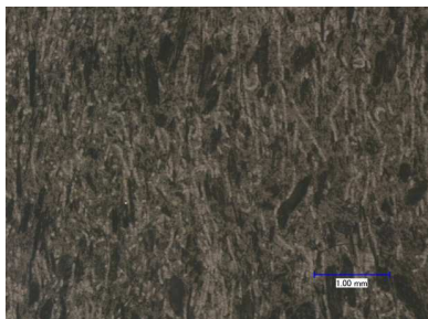
Figure 6: Incident Light Microscopy PP + 40% wood + 10% PET fibers + 5% bonding agent; resolution 50x
