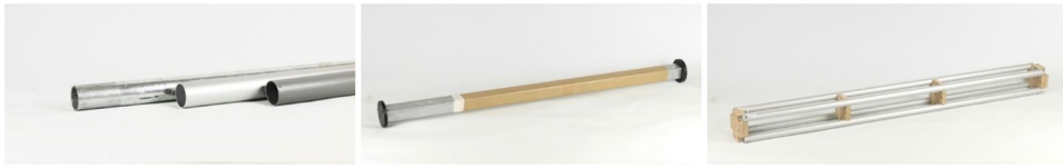
Fig. 7 Left, middle: as formwork, we tested steel, aluminum and plastic profiles of both circular and rectangular cross-sections of 40 and 50 mm diameter. Right: for larger rectangular cross-sections, a form-
