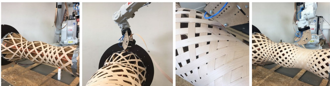
Fig. 10 Left: rib formwork, composed of a series 5 mm MDF plates that were CNC milled according to the surface design. At both ends, rings provide the precise spacing distance. Middle, right: fabrication of a 1200-mm-long customized component, with a varying diameter of 224–518 mm component with 28 winding lines. We used an ABB
