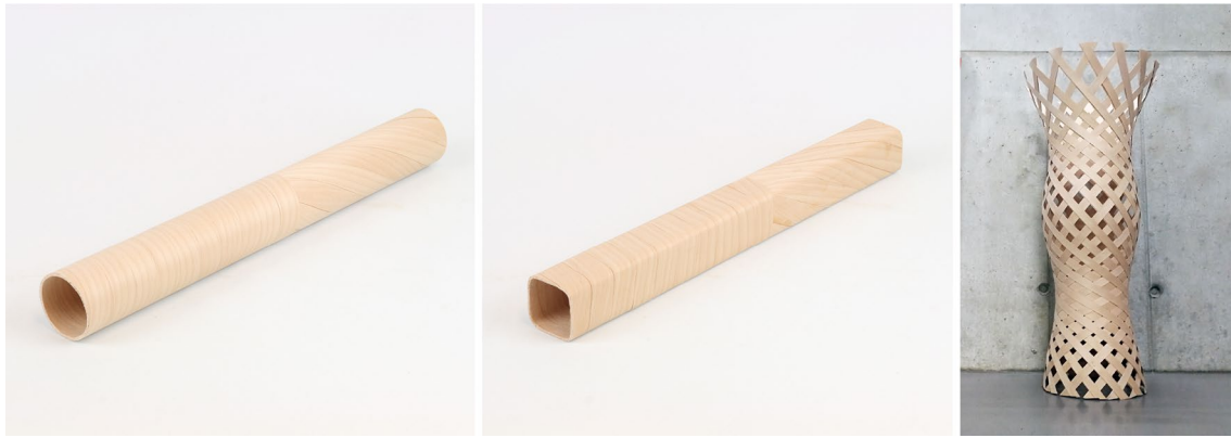
Fig. 13 Case study prototypes of robotically wound components. Left: round profile with 7 layers of beech veneer. Middle: square profile with 7 layers. Right: free-form rotational surfaces with 4 layers
