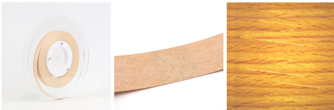
Fig. 1 Left: 24×0.5 mm beech veneer filament, on a custom spool. Middle: cellulose fleece coating on the back of the veneer. Right: close-up of finger-joint of veneer strips
