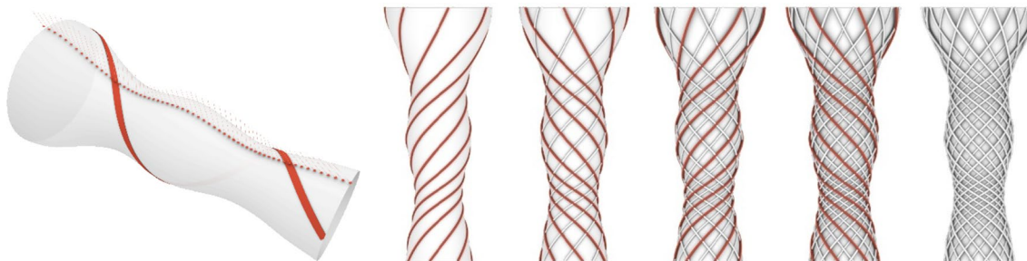
Fig. 9 Left: rotational surface with free-form section. Right: winding lines generation, to create an effect of braiding: 1st layer: 7 cw, 2nd layer: 7 ccw, 3rd layer: 7 cw (50% shifted), 4th layer: 7 ccw (50% shifted)
