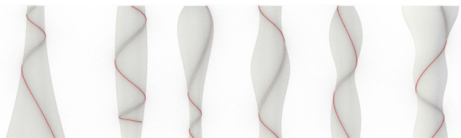
Fig. 12 Results of the generation of winding lines based on local geodesic curves on a range of different free-form rotational surfaces
