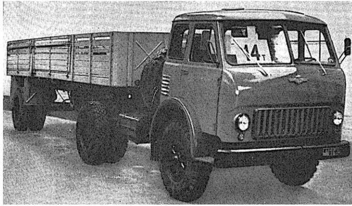
LKW KAS 504, 14 tons capacity from Kutaissi Automobil Works in Georgian SSR, (Source: Automobilpraktiker, 1966, issue 4, p. 19)
