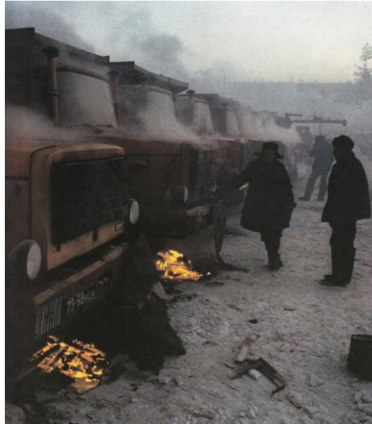
Figure 1: Keeping truck motors warm in the winter in the Soviet Union in 1980
