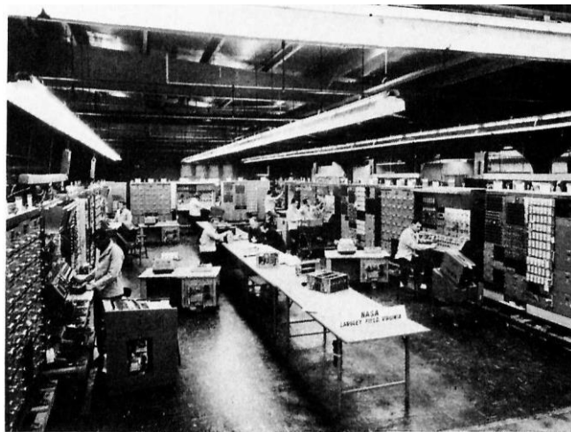
Figure 15: Analogue Computer EAI 231R prepared for Langley's computing center in 1961 93
