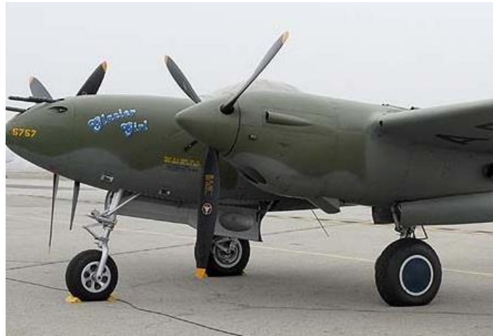
Figure 12: Landing Gear of Lockheed P-38 (Press Release Lockheed)
