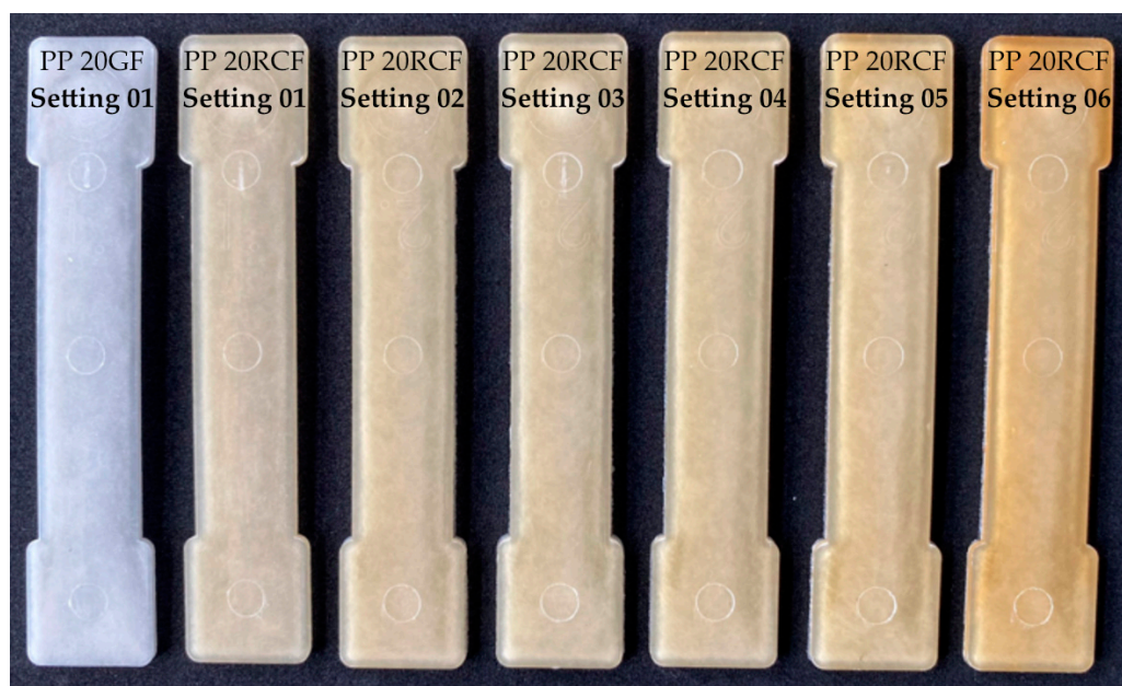
Figure 5. Representative specimens of PP 20GF (Setting 01) and PP 20RCF (Setting 01 to Setting 06).
