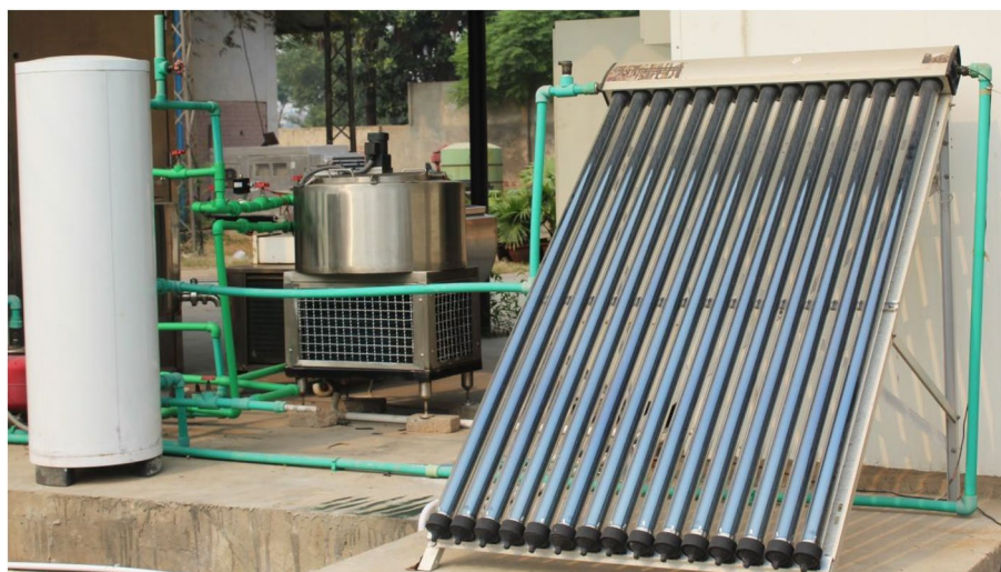
Figure 1. Solar assisted yogurt processing unit 20 .
