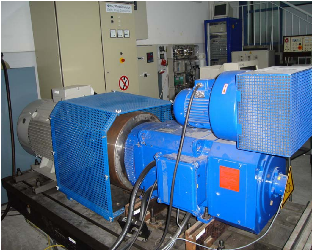
Figure 27: Grid Simulator at DeMoTec laboratory
