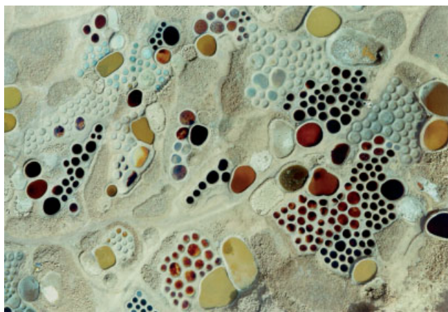
Figure 1: Aerial photograph of the evaporative salt-enrichment ponds at the Teguidda-n-Tessoumt salt mine, Niger, West Africa. The photograph was taken from 150 m height using a simple kite-based system (Buerkert et al., 1996).
