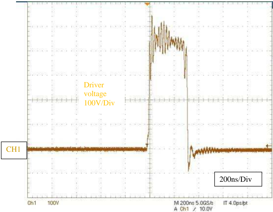
Fig. 62: Output voltage of the gate driver with load (CH1: driver output voltage)
