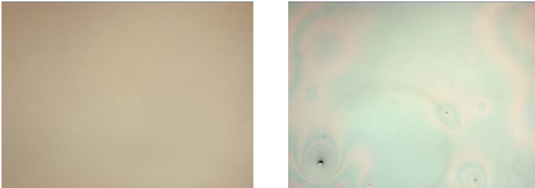
Figure 5.11: Coating process of PAK-01 polymer, the surface looked homogeneous with adhesion promoter TI-Prime (left), and with mr-APS1 (right) where the inhomogeneity of the surface showed different colors.
