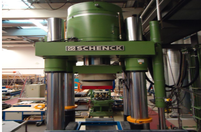
Fig. 3.8: Testing machine and hydraulic jacks
