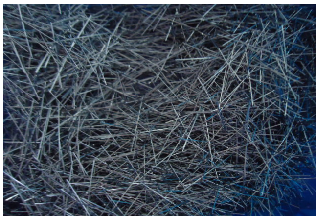
Fig. 3.3: Steel fiber used in constructing the specimens
