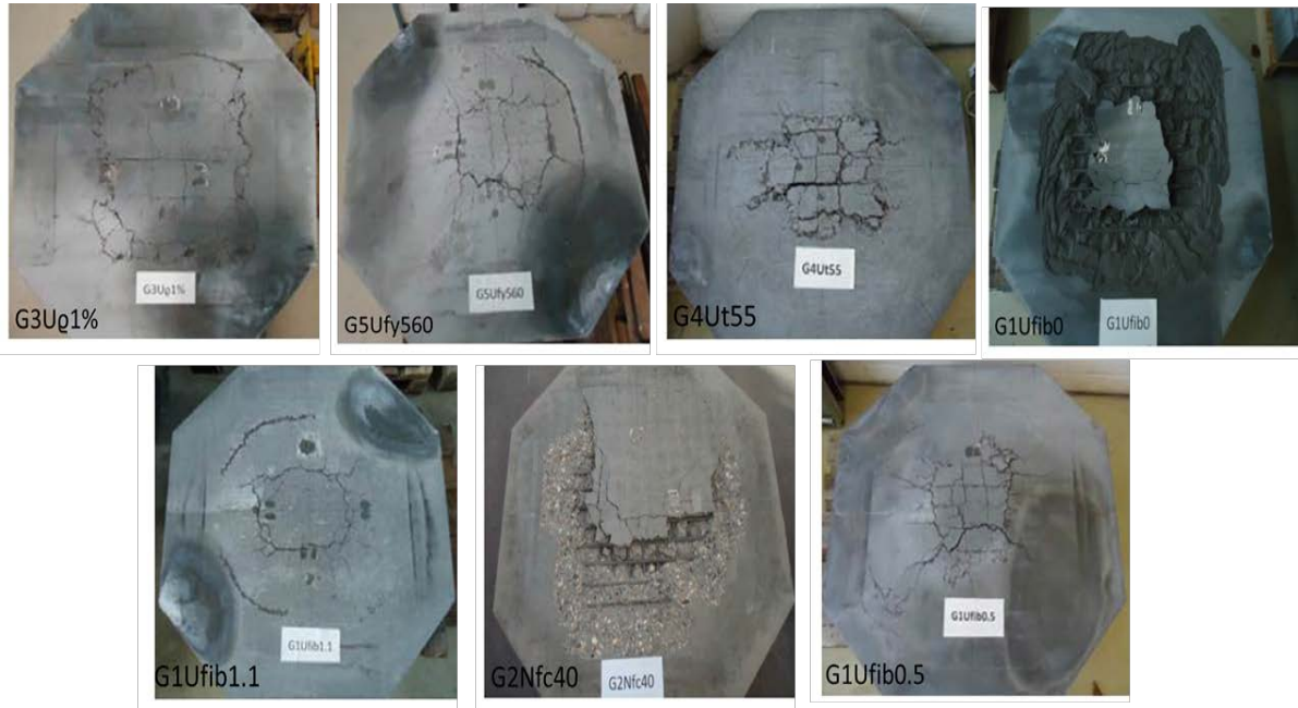
Fig. 4.3: Tested slabs' modes of failure
