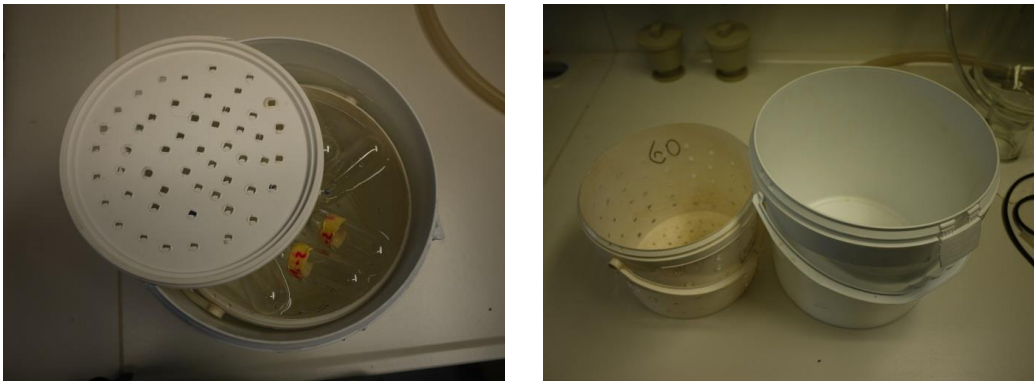
Figure 1.2: Water filled transportation bucket for gas sampling tubes
