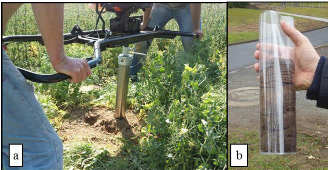
Fig. S3 (a) HUMAX, a special soil sampling drilling tool (b) The soil will be automatically filled in a plastic cylinder.
